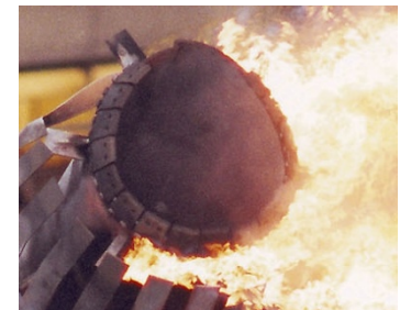
Missing Flame Retention Lugs & Cracked Body at 12 o/c
