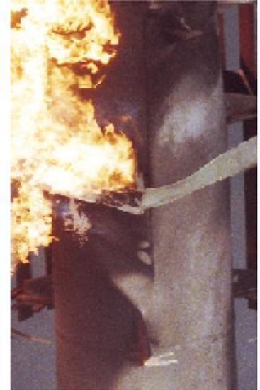
Visible Crack in Flare Body
